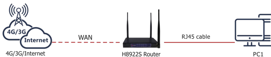
Figure 3-3 Single Equipment Direct Connection
