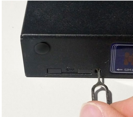
Figure 3-1 Pop out SIM slot
